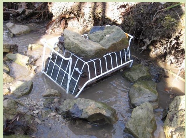
The prototype consists of a dishwashing rack lined with window mesh with tempered hardboard inside. Photo, Meg Maloney
